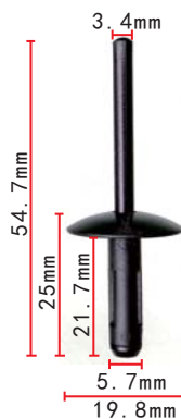
C1986 Nylon Original Front Bumper Retaining Grommet Nissan#01281-01431
