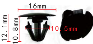
C1936 POM Black Mud Guard Extension Panel Retaining Clip Toyota#90467-06192
