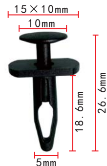
C1408 Nylon Black Push-Type Retainer VW
