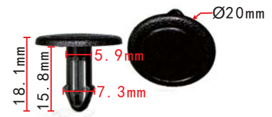
C1952 POM Black Engine Compartment sides/ Dashboard Retaining Clip Honda#91501-SNA-003
