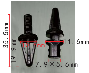
C1768 POM Black Rear Bumper Retaining Clip Nissan 85284-7S610
