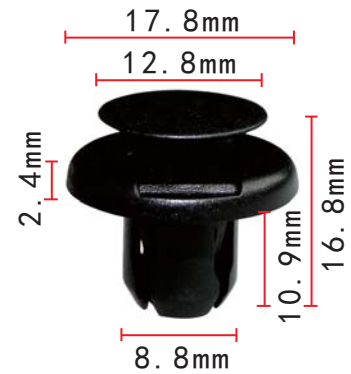
C997 POM Black Vent Cover Push-Type Retainer Toyota Hiace
