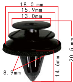
C1129 POM Black Door Inner Liner Retainer Nissan 84953-AU100,80999-VE000
