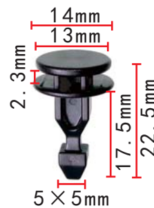
C3165 Nylon Black Door Sealing Strip Clip Honda#90651-TG7-000
