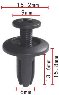
C91 Nylon Black Front Fender Rocker Panel Push-Type Retainer Prelude; Nissan
