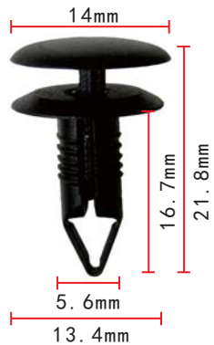
C574 Nylon Black Interior Trim Push-Type Retainer Ford; Mazda
