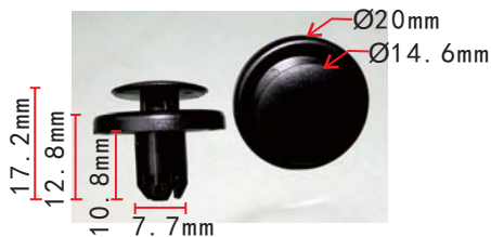
C1876 POM Black Fender Liner Retainer Clip SUBARU 909140068
