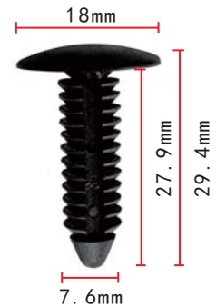
C582 Nylon Black Shield Retainer Battery Post Cable Shield, Engine Splash Shield Radiator Side Air Baffle GM; Chrysler; Ford 390018-S
