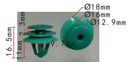
C3042 POM Green Front Door Trim Panel Retaining Clip Hyundai#82315-2W000
