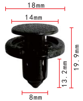
C351 POM Black Bumper Clip Push-Type Retainer Nissan 01553-09611, 01553-10501, 90467-08185
