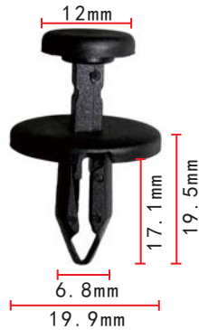
C831 Nylon Black Side Radiator Shield Push-Type Retainer Chrysler 6506132-AA
