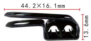
C1209 POM Black Routing Clip With Iron Shield Toyota Alphaard
