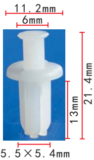
C251 Nylon White Push-Type Retainer Mercedes-Benz
