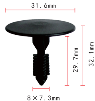
C208 Nylon Black Interior Trim Retainer Ford 1986-On N804349S
