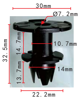
C1589 POM Black Rocker Panel / Lower Side Sill Retainer BMW
