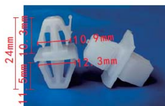
C1824 POM White Side Sill & Windowsill Trim Retaining Clip VOLVO 30808521
