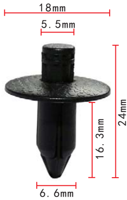
C189 POM Black Push-Type Retainer Nissan; Toyota; Suzuki; Mitsubishi
