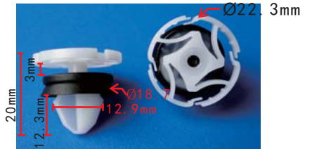
C1761 POM White (with washer) Door Inner Trim Panel Retaining Clip Renault 7703077476 ; Peugeot Citroen 9345.ZN
