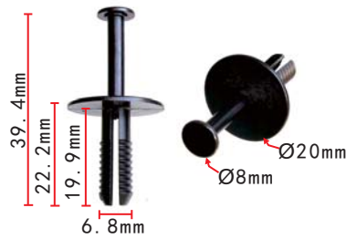
C1999 Nylon Black Front Bumper Retainer GM#90508809,1400806
