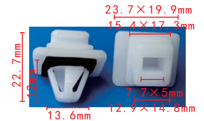
C1523 POM White Door Anti-Collision Strip Retainer Honda 90501-S9A-003
