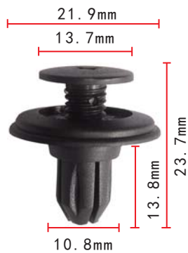
C70 Nylon Black Bumper & Fascia Push-Type Retainer Nissan 1986-On 01553-03101
