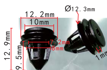
C1640 Nylon Beige & Black Door Trim / Bumper / Luggage Cover Nut Rod Diameter: 8.4x8mm VW N10516801 BMW 51127020321; Audi
