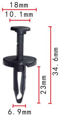
C47 Nylon Black Body Retainer GM 20510029; Ford N803362-S Chrysler 34202672
