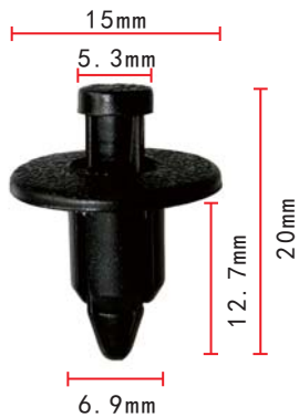
C564 POM Black Push-Type Retainer GM 96057846 , Toyota 90467-07041 Suzuki 09409-07308-5PK
