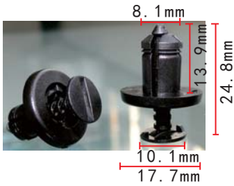
C1549 POM Black Bumper Grille Retainer Renault 7703072360
