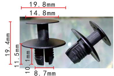
C1679 Nylon Black Grey Hood Insulation Retainer Mercedes-Benz
