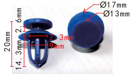
C1767 POM Blue Door Trim Panel Retaining Clip GM 13252118 Opel 7231991
