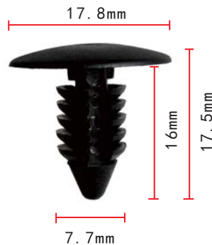
C413 Nylon Black Fender & Bumper Shield Retainer GM; Ford; AMC; Chrysler
