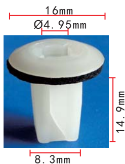
C286 Nylon White Grommet #10 Screw Size
