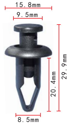
C121 Nylon Black Body Side Moulding Push-Type Retainer Nissan 76882-57A00
