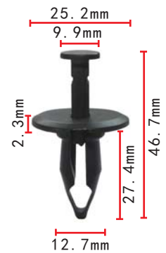
C160 Nylon Black Bumper Fascia Retainer GM 1987-On 10053388, 22542705
