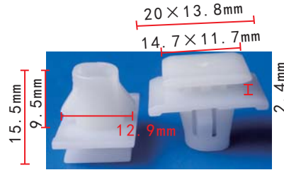
C1614 POM White Rocker Panel Retainer Honda 75315-S9A-004
