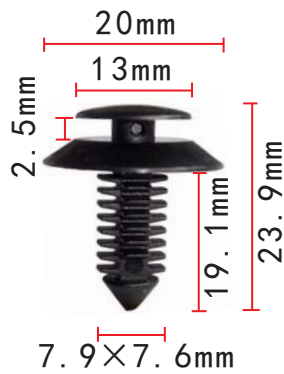
C8 Nylon Black Door Trim Panel Retainer Ford N801925-S
