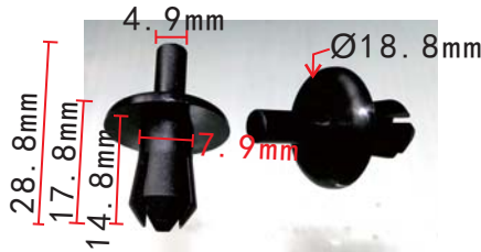
C1763 POM White (With Rubber) Door Trim Panel Retaining Clip Peugeot 6991Y8 Fiat 9654280780 Renault 7703077469
