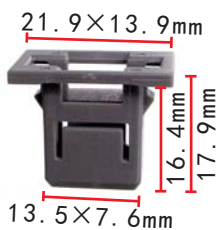
C3161 POM Dark Brown Engine Cover Latch/Front Grille Retaining Clip Honda#91548-TZ5-A02
