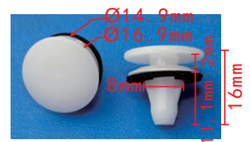
C1967 POM White Rear Combination Light Retaining Clip Hyundai#92485-2H000
