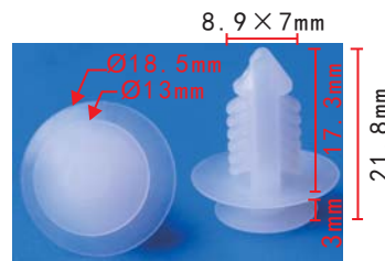
C1616 POM Yellow Trunk Rack Trim Retainer Toyota 90467-09198
