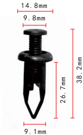
C641 POM Black Bumper Cover & Wheel Housing Push-Type Retainer Toyota 90467-09139
