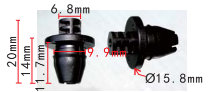
C1874 Nylon Black Fender Retainer AUDI#8K0-868-307
