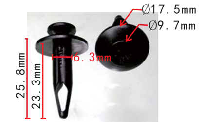
C1774 Nylon Black Side Sill Panel Retaining Clip Ford W705848S300
