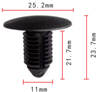
C626 Nylon Black Weatherstrip Retainer Chrysler 4658673
