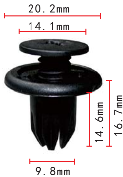
C570 Nylon Black Front & Rear Bumper Push-Type Retainer Honda ; Subaru ; Mini
