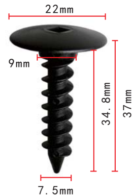
C642 Nylon Black Foam to Bumper Fascia Screw Ford 6503819, 6503401 Chrysler 1993-On
